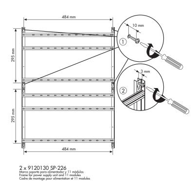
CÓMO FIJAR EL COFRE EN LA PARED HOW TO FIX CABINET ON THE WALL COMMENT FIXER LE COFFRET SUR LE MUR CÓMO CERRAR EL COFRE HOW TO CLOSE CABINET DOOR COMMENT FERMER LE COFFRET
