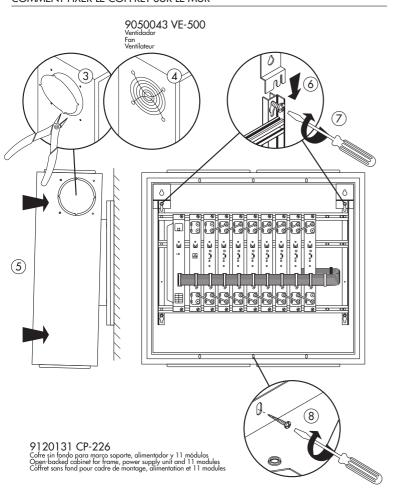
COTAS DE POSICIONAMIENTO DEL MARCO SP-226 Y DEL COFRE CP-226 RACK MOUNTING PLAN FOR SP-226 FRAME AND CP-226 CABINET COTES DE POSITIONNEMENT DU CADRE DE MONTAGE SP-226 ET DU COFFRET CP-226
